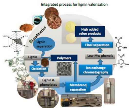
Figure 1. Integrated process for lignin valorization
